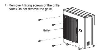
Insert the support A between the outdoor unit and the grille, and reinstall the screws that removed in 1).
