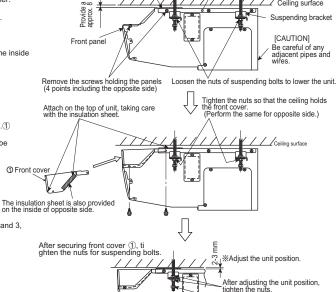
Insulation sheet on top of unit
