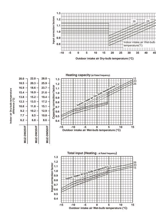
**NOTE:** The above broken lines are for the heating operation without any frost and defrost operation.
