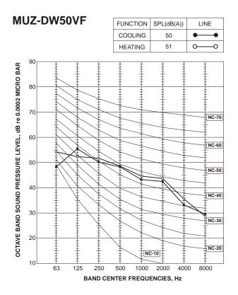
Test conditions Cooling: Dry-bulb temperature 35°C Wet-bulb temperature 24°C Heating: Dry-bulb temperature 7°C Wet-bulb temperature 6°C
